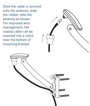
At this point, please determine the best way to route the rest of the cable into your home to the XM home receiver or XM Plug & Play system.
